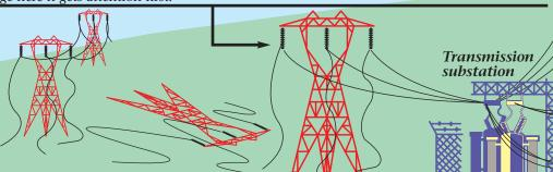
**Step 2.** A co-op may have several local distribution substations, each serving thousands of consumers. When a major outage occurs, the local distribution substations are checked first. A problem here could be caused by failure in the transmission system supplying the substation. If the problem can be corrected at the substation level, power may be restored to a large number of people.
